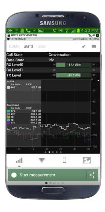
Xpedite Hand Held Tester is used to measure and collect data that is critical for system operators, engineering, customer support, cell site maintenance and repair, as well as wireless consultants.
